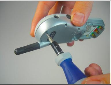
Using the Torx T4 screwdriver remove the six screws highlighted in the picture to the left
