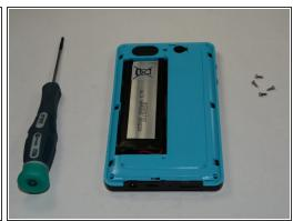
To remove the battery, make sure the four 5mm Philips screws on each side of your device is open using the Phillips #1 Screwdriver.
