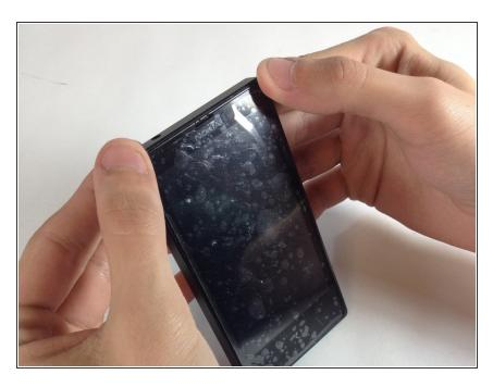
The first step is to remove the back cover off of the phone. To do this, place both your thumbs on the two top corners of the device and simply pop it off.
