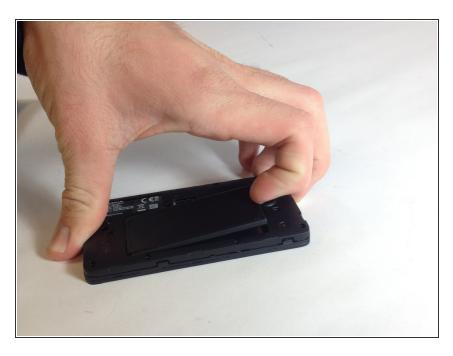
To remove the battery, simply use your finger to pry the battery out of its slot.
