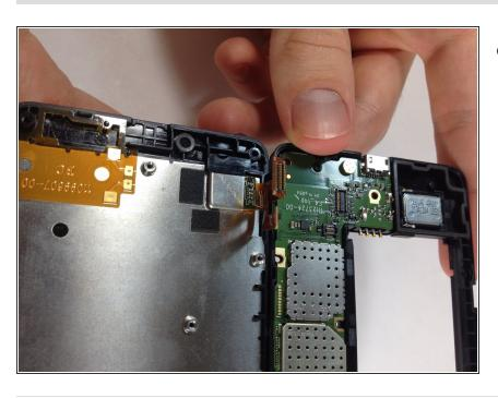
If the connectors are still attached, simply unhook them by lifting the top of the connector with your finger.
