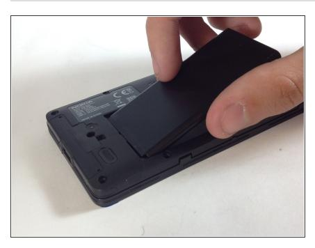
Inserting a new battery is as simple as lining up the gold connectors and sliding the battery in text-side down.
