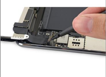
• Use spudger to lift the LCD connector up off its socket on the logic board.
