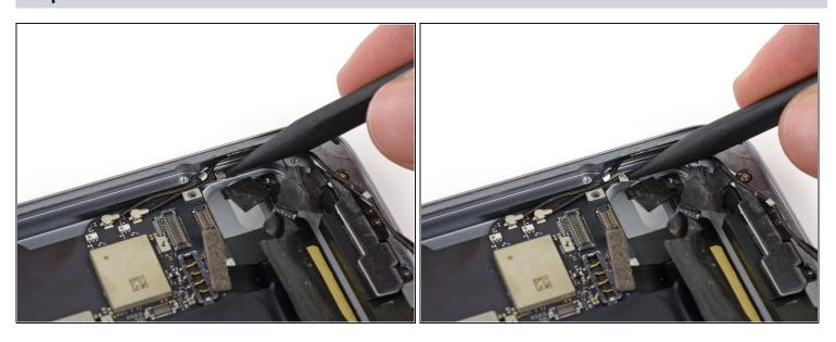
Use the point of a spudger to pull the antenna cable clip toward the battery to allow access to the cables.
