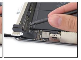
Use the flat tip of a spudger to gently lift the battery connector up off its socket on the logic board.
