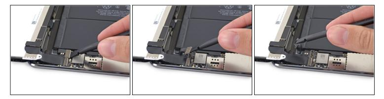
• Use the flat tip of a spudger to gently lift the battery connector up off its socket on the logic board.
