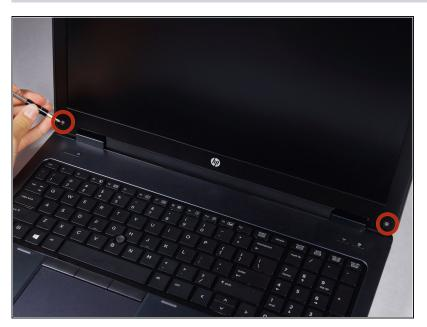
Remove the two 6mm screws with a Phillips #0 screwdriver.
