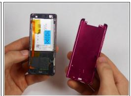
Remove the back plate from the device.
