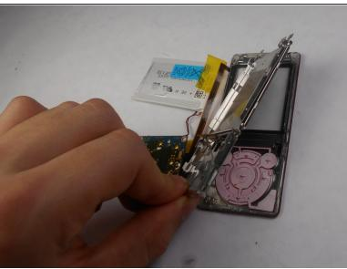
Disconnect the metal shielding plate from the front panel with tweezers or a plastic opening tool.
