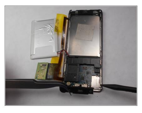
Use a nylon spudger or tweezers to remove the plastic USB cover.
