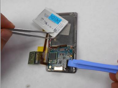
Use a Phillips #00 screwdriver to unscrew two 2 mm screws, and remove the motherboard from the device with tweezers and a plastic opening tool.
