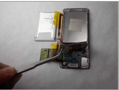
Remove the plastic protective frame located over the motherboard with tweezers and a spudger.
