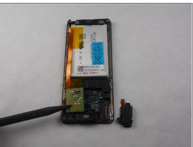
Disconnect the headphone jack connection from the motherboard using any tool to remove black audio piece that needs to be replaced.
