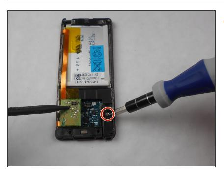
Unscrew one 2.5 mm screw using a Phillips #00 screwdriver on bottom right portion of device located near audio jack.
