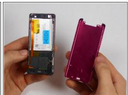
Remove the back plate from the device.
