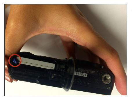
There is a small blue tab on the right of the compartment. In order to remove the battery, move this tab aside and the battery will pop up.
