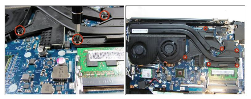
• Remove all six 7mm screws from the heat sink using the Phillips #1 screwdriver.
