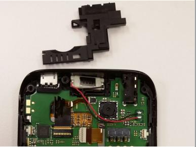
Grab the housing on the bottom left side with fingers and pull outwards and towards the bottom of the phone.
