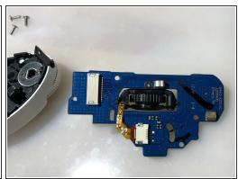
Make sure the dial slot aligns with the power switch board prior to reassembly.
