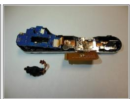
The jog dial should fall out easily. If not, use a pair of tweezers to gently poke it though the power board.
