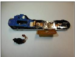
• The jog dial should fall out easily. If not, use a pair of tweezers to gently poke it though the power board.
