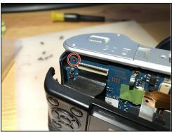
• Using a Phillips #00 precision screwdriver, remove the 3mm screw holding the top panel of the camera in place. Also, remove the screws under hot shoe metal clip, otherwise you can break a piece of sensor frame leading to costly repair.
