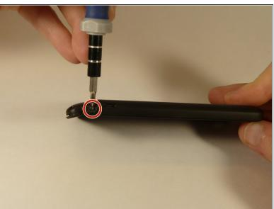
Remove the 2.0 mm Phillips #0 screws on either side of the phone.
