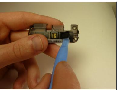
Using a plastic opening tool, peel off the speaker cover.
