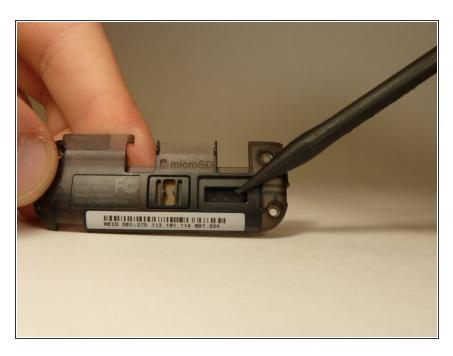
Use the spudger to push the speaker out of its casing.
