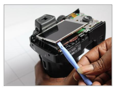
Fold the LCD screen back into the proper position.
