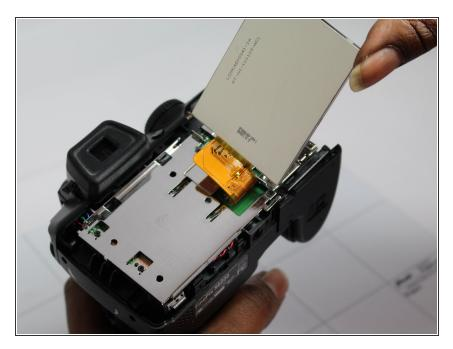
Fold back the LCD screen and check that the cable coming from the screen is securely fastened to the motherboard.
