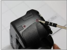
Remove the 4mm JIS #00 screws from the sides and bottom of the camera.
