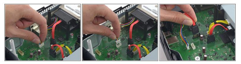
• Disconnect the hard drive SATA power and data cables from the motherboard.
