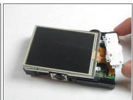
Remove the three 5 mm screws
