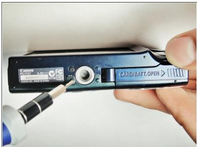
Remove the two 5.00 mm screws in the bottom of the casing with a Philips #000 screwdriver
