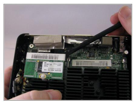
Using the spudger, gently push on the underside of the memory board to loosen it. Gently grasp each side and pull up to release the memory board.
