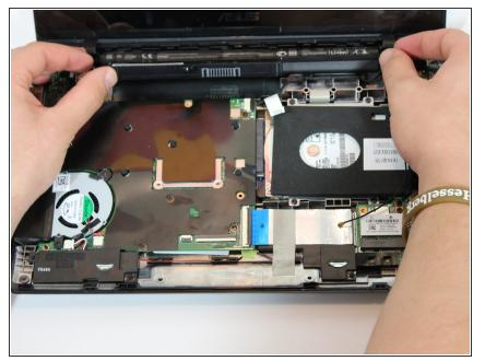
• Slide the battery up and out.
