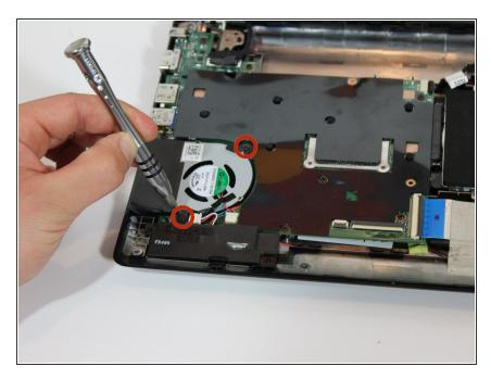
Remove the Two 4 mm screws using Phillips #0 phillips screwdriver.
