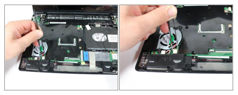
• Unplug the set of wires located at bottom corner on fan.
