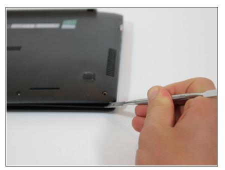
Use a plastic or metal spudger to separate the keyboard from the back panel and lift the keyboard out of place.
