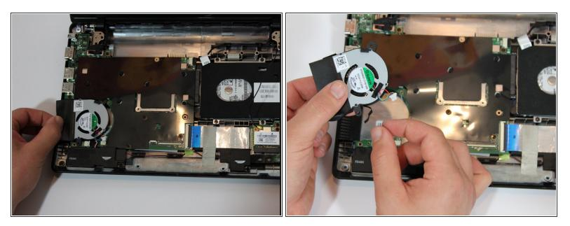
• Lift up and out to completely the remove fan component.
