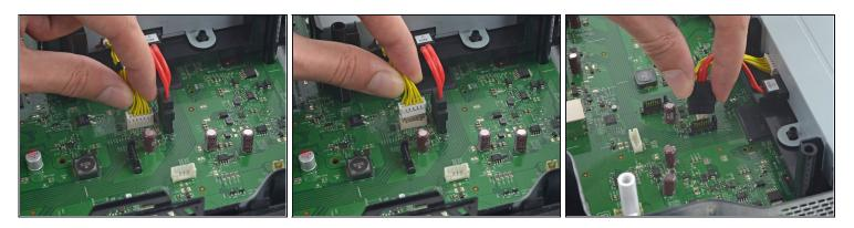
• Disconnect the optical drive power and SATA data cables from the motherboard.
