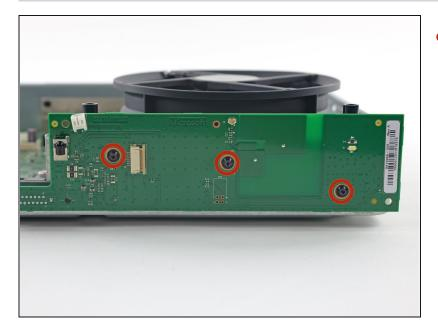
Remove the three 9.5 mm T9 Torx screws securing the front panel board.
