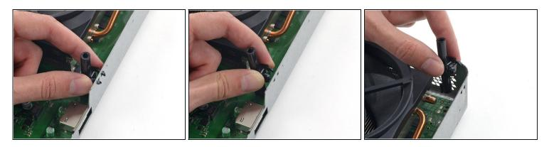
*i* Two black plastic screw posts posts are attached to the frame with springy plastic barbs.
