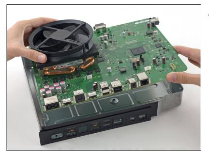
• Lift the motherboard and heat sink/fan assembly out of the lower metal case.
