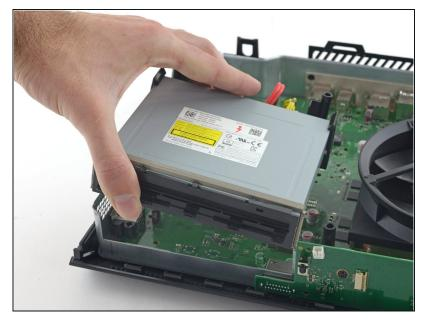
• Remove the optical drive assembly from the Xbox.
