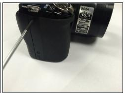
On the left side of the camera, remove two screws using a Phillips #00 screwdriver.
