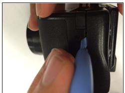
Use a plastic opening tool to gently loosen up the sides of the camera.
