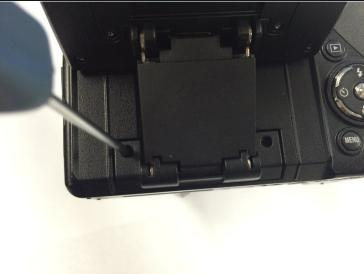
Remove the two screws hidden underneath the display panel.
