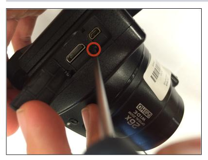
Lift the HDMI and A/V OUT cover to access the hidden screw.
