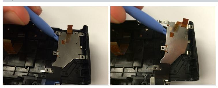
• Use a plastic opening tool to lift the metal plate and set it aside.
