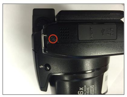
• On the right side of the camera, remove the first visible screw.
