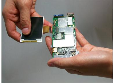
Carefully grip the screen and pull it away from the ribbon connector located on the motherboard.
