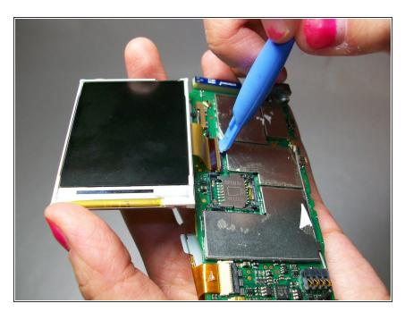
Gently lift the latch on the the ribbon cable connector inward (towards the motherboard).
