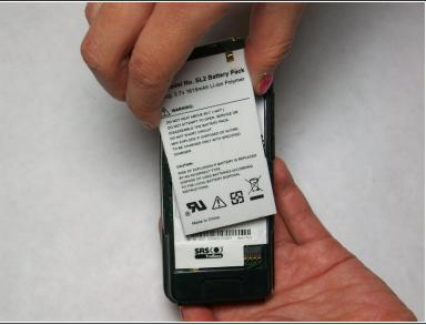
Pinch the battery from both sides and lift the battery to remove it.
