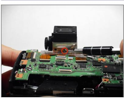
Using a Phillips #000 Precision Screwdriver, remove the 3.0 mm screw that holds the eyepiece in place.
