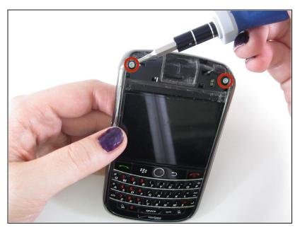
Use the T6 Torx screwdriver to remove the two 8.00mm screws from the top of the phone.
