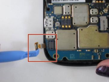
• Using a small opening tool, pry up the pop ribbon cable from the motherboard.
