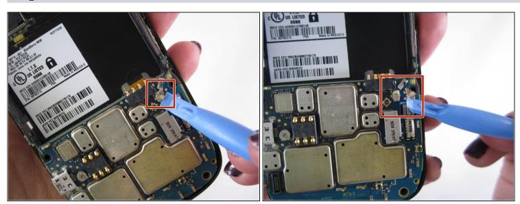
Using a small opening tool, remove the side antenna cable.
