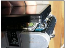
Place a plastic opening tool into the gap between the back panel and camera body, from both the top and the bottom of camera. Carefully pry open the camera and separate the back panel.
