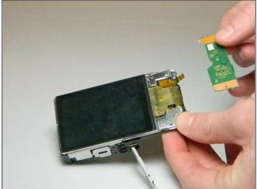
• Flip over the control board then use <u>tweezers</u> to pull out the ribbon connecting the circuit board to the motherboard.
