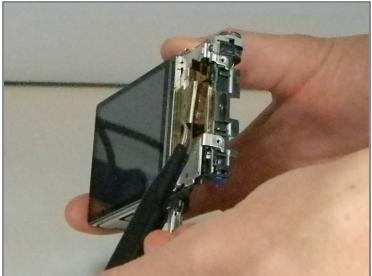
• Use <u>tweezers</u> to remove the ribbon that is connected from the LCD screen to the camera by pulling the part that is folded under, out.
