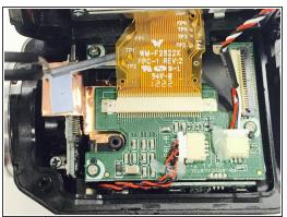
Using the tweezers, carefully push up the left and right sides of the cable ribbon clip. Use the tweezers to life up and remove the clip.
