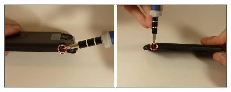
• Remove the 2.0 mm Phillips #0 screws on either side of the phone.
