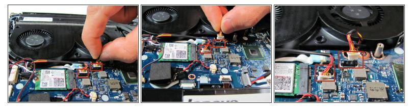
Pull the wire tabs up one at a time to separate them from the motherboard.
