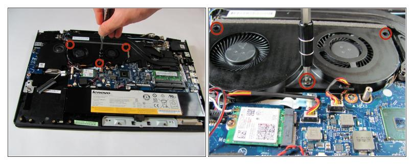
• Remove the three 3.5 mm screws from the fan with a Philips #1 screwdriver.
