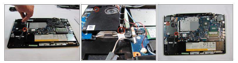
• Using a Philips #1 screwdriver, remove the two 2.5 mm screws securing the bass speaker.
