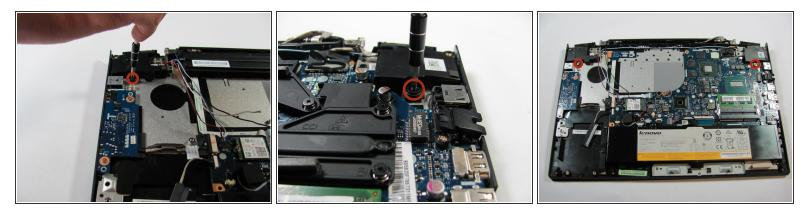
Using a Philips #1 screwdriver, Remove the 2.5 mm screw holding each side speaker to the laptop.
