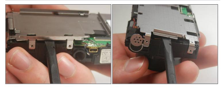
• Pry the metal plate out using the spudger.
