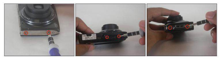
• Unscrew the six 3.5mm Philips head from the outer casing.
