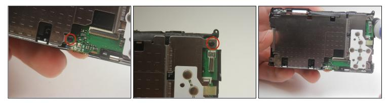
• Unscrew the two 3.5 mm Phillips head screws in the metal plate.
