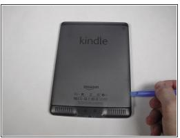
Use the plastic opening tool to undo the ten plastic clips around the back panel of the Kindle.
