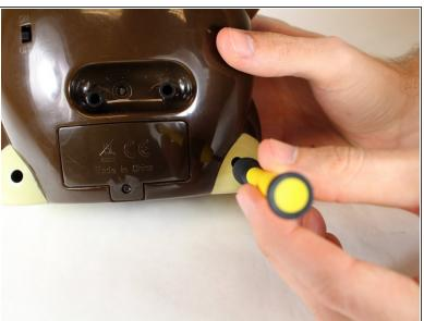
Remove all six 7.3 mm screws with a #00 Phillips head screwdriver.
