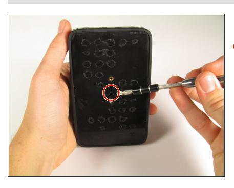
Remove the one 4.5 mm Phillips #0 screw on the back panel of the mixamp.
