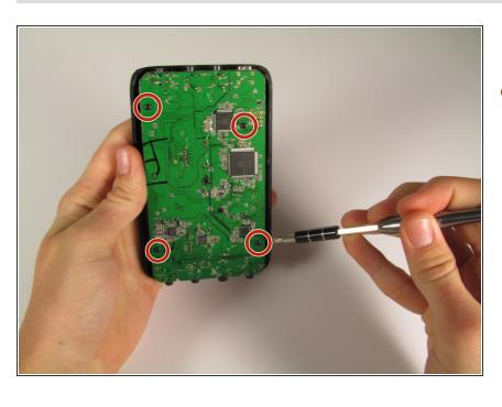
Remove the four 5.8 mm Phillips #0 screws on the motherboard.
