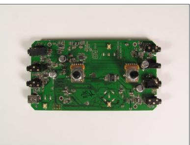
Remove the motherboard from the casing.
