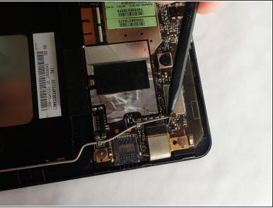
Pry the GPS Antenna cable straight up using a spudger or similar prying tool. It will be the grey
