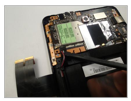
Locate the speaker wires to the left side of the battery. Remove the connector by pulling up gently or prying with a tool if you can not get a good grip.
