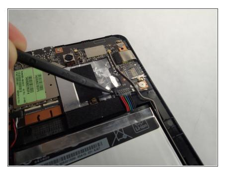
Locate the battery connector by following the wires that come from the top right of the battery. To disconnect the battery just lift up gently on the wires. Use a spudger or blue plastic opening tool to gently lift the wires if it is hard to get a grip.
