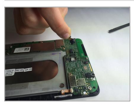
Remove the camera from the device.
