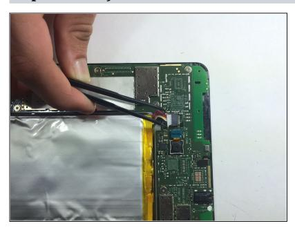
Gently disconnect the battery from the motherboard using your fingers or a pair of tweezers.
