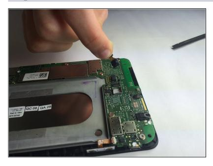
Remove the camera from the device.
