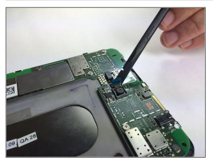
• Use a spudger to disconnect the camera from the motherboard.
