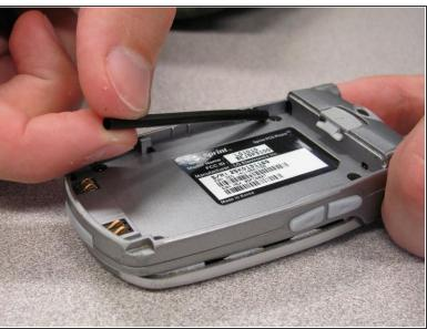
Pull the antenna housing (black tube) towards bottom of phone and remove.
