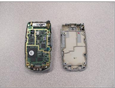
Pull the back cover straight off the phone using your thumb and forefinger.
