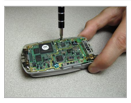
Pry off circuit board with a flathead screwdriver.
