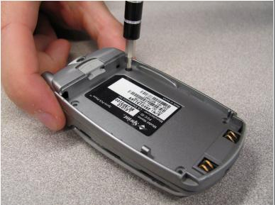
Unscrew the four screws on the back case using a T6 Torx Screwdriver.
