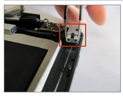
• Use <u>tweezers</u> to carefully remove the charger port cover.
