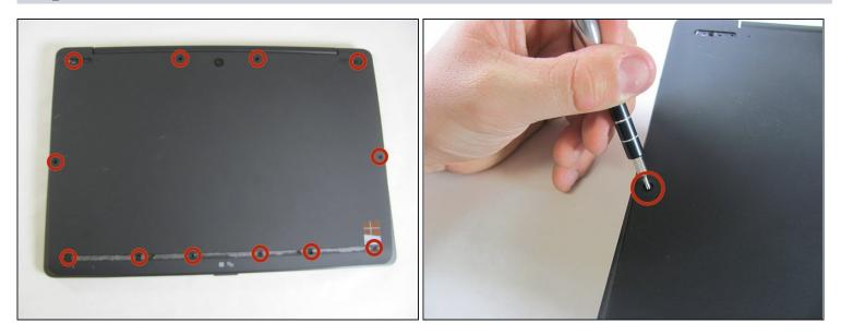
• Starting with the laptop top-down, locate and remove the twelve 1mm Phillips #0 screws securing the back cover to the main body of the computer.
