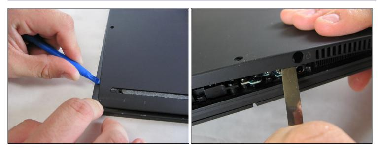
• Use the Plastic Opening Tools or Metal Spudger to carefully loosen back cover from the body of the computer.
