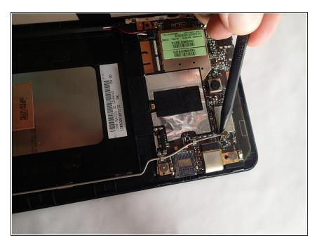
Pry the GPS Antenna cable straight up using a spudger or similar prying tool. It will be the grey wire that runs up the right side of the device coming from the speaker housing up to the motherboard.
