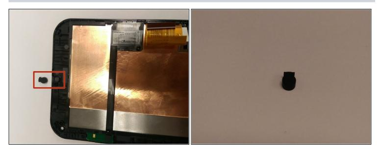
*i* The screen has a rubber device used to support the volume control switch.
