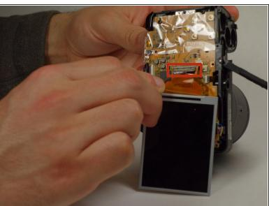
Disconnect the ribbons that connect the LCD screen to the camera gently using precision tweezers or fingers.
