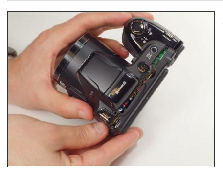
Carefully detach the back side of the camera by lifting both ends, with moderate force wobble until loosened enough to remove.
