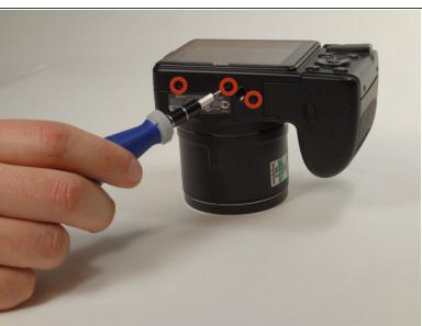
Remove three 5 mm Phillips #000 screws on the bottom end of the camera.
