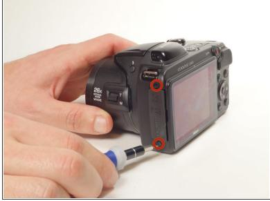
• Remove two 5 mm Phillips #000 screws near the audio/video inputs on the opposite side near the flash component.
