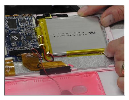
Once the device is open, remove the tape from the the battery.
