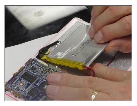
Remove all tape connected to the battery.
