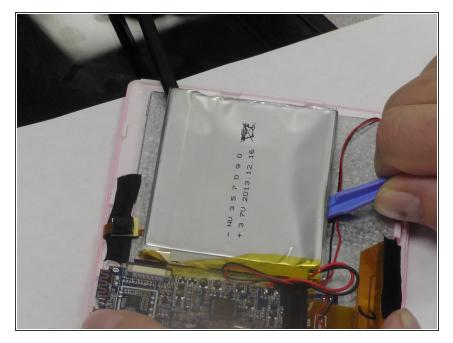
Carefully pry up the battery by wedging the plastic opening tool under the battery. It is glued to the screen so it will be a delicate removal process.
