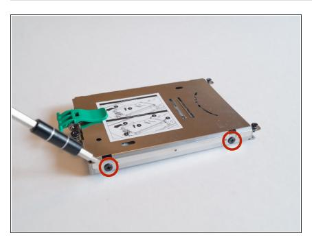
Remove the two 3mm screws on either side of the device with a Phillips #0 screwdriver to remove the drive caddy.
