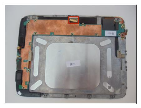
Disconnect the gold connector by lifting the latch with the plastic opening tool.
