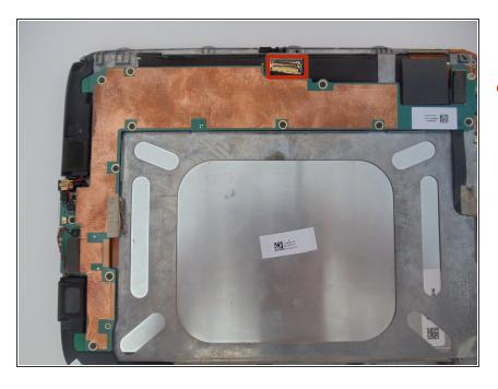
First Disconnect the gold connector by lifting the latch on it up and pulling it loose using the latch to pull.
