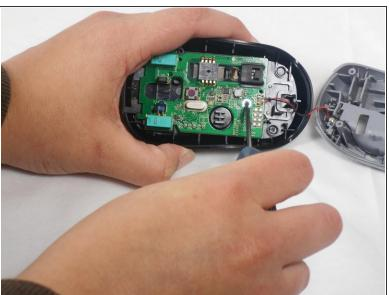
• Unscrew the 0.25mm phillips head screw to release the circuit board.
