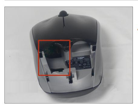
Remember to insert the new battery in the same orientation as the old one. The positive (plus) end should be facing away from the buttons.
