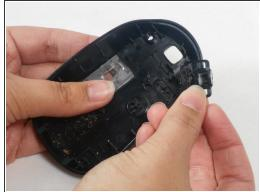
• Unscrew the 0.25mm phillips head screw holding the button in place. The cover release button can then be removed.
