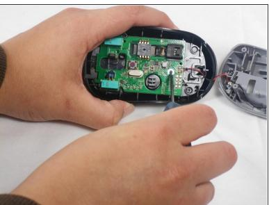
Unscrew the 0.25mm phillips head screw to release the circuit board.
