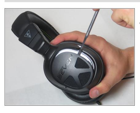
Apply a gentle pressure outward so that the side plate will pop off. To put the side plate back, simply snap the side plate into place.
