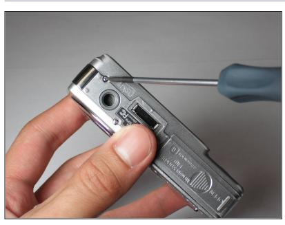
Remove the screw using the Phillips #00 screwdriver from the bottom of the camera, closest to the back cover.
