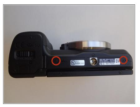
Remove the two 3.5mm Phillips #00 screws that hold the back case located on the bottom of the camera.
