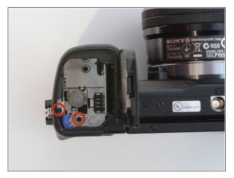
Remove the two 3.5mm Phillips #00 screws that hold the back case located inside the battery compartment.
